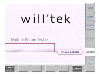
In the Welcome screen, you can immediately start testing GSM mobiles in call mode by pressing the **Calls & Meas.** softkey below the TFT display.
