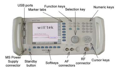
**Standby button** This button switches the 4400 from stand-by mode to operating mode. The light below the button lights yellow in stand-by mode and green in operating mode.
