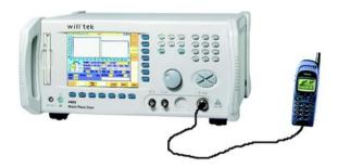
**Off-air** With an off-air connection, the RF socket of the tester is connected connection to Willtek's Universal Antenna Coupler. This makes testing easy and fast. The mobile transmits via the antenna. No further test adapters are needed.
